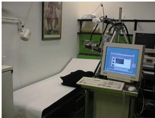
The first generation PPGI system in examination rooms of the University Hospital Aachen in a study for contactless functional quantification of skin perfusion
