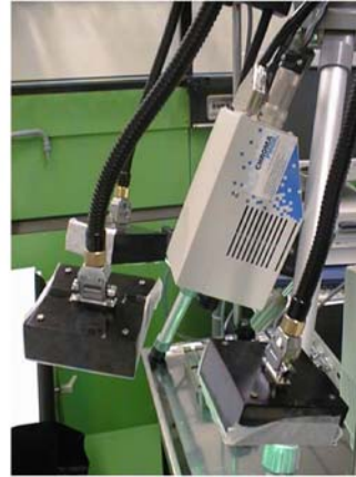
The first generation PPGI system in examination rooms of the University Hospital Aachen in a study for contactless functional quantification of skin perfusion
